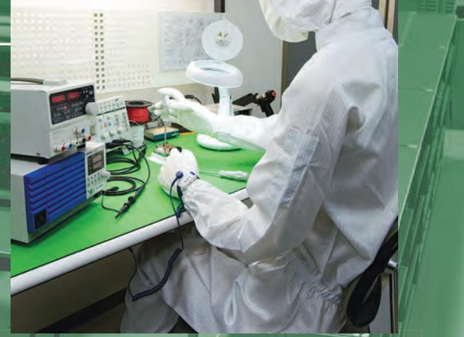
We provide IEC standards-compatible ESD protection items ranging from EPA working mats laid on workbenches, storage racks, and trolley surfaces, EPA flooring for PVC floors or floor coating, and to wrist straps for ESD countermeasures.
