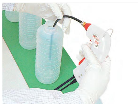
Static electricity removal in a bottle
