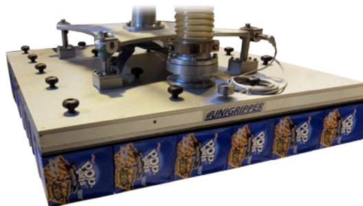
Almost all LayerGrippers are equipped with the floating attachment, and, depending on the products to handle, side clamps with or without side skirts.
