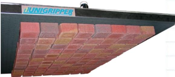
100% customized to each project, we build the UniGripper Customized to our well proven standard. The unique patented valve technology allows the Gripper to literally recognize if and where a product is located underneath it, and applies vacuum to the product only.
